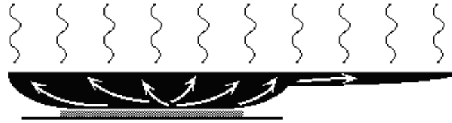
Figure 5. Heat conducted through the pan to handle
