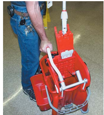
Certain types of microfiber mops require much less force to squeeze the mop dry.
